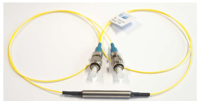
Alternative configuration – Bragg-mirror coated on the fiber end, butt coupled to another fiber, and mounted in a steel tube.
