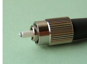
figure 2: same connector as figure 1 with heat conducting paste
