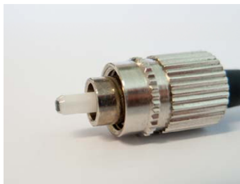
RSAM chip on FC/PC connector end face
