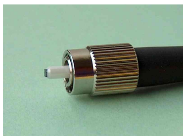
Figure 1: SAM chip on FC/PC connector end face
