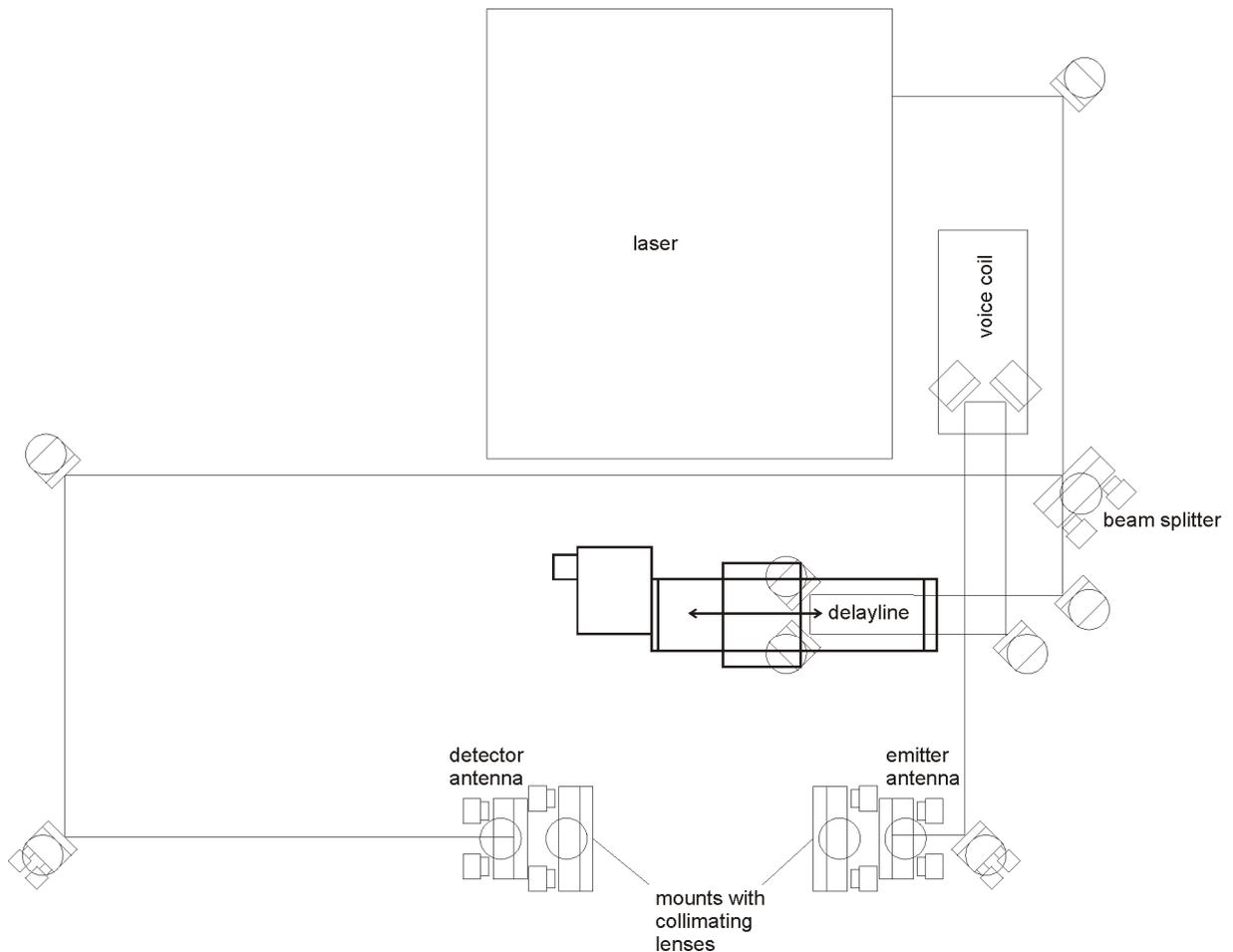
2. Position all elements loosely on the bread board and measure the distances in order to make sure that the path lengths add up (as described in the manual for building your own THz setup)
