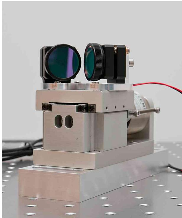
The Fast Scan Unit consists of a voice coil, an electronics box and a few cables to connect them with each other. Additionally, there is one coaxial cable that needs to be connected to the National Instruments Data Acquisition Unit (DAQ). Otherwise, the T3DS software will not be able to display the THz signal correctly.
