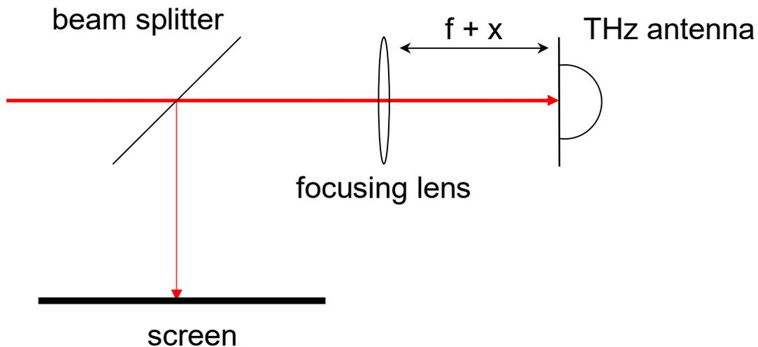
An alternative set-up using a screen with a hole for the laser beam is shown below:
