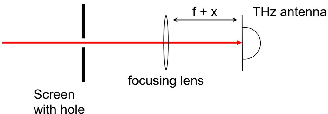
According to the thin lens formula  $\frac{1}{f} = \frac{1}{S1} + \frac{1}{S2}$  the image will be visible on a screen in a distance  $S2$  from the lens. ( $f$  – focus length,  $S1$  – object distance,  $S2$  – image distance)
