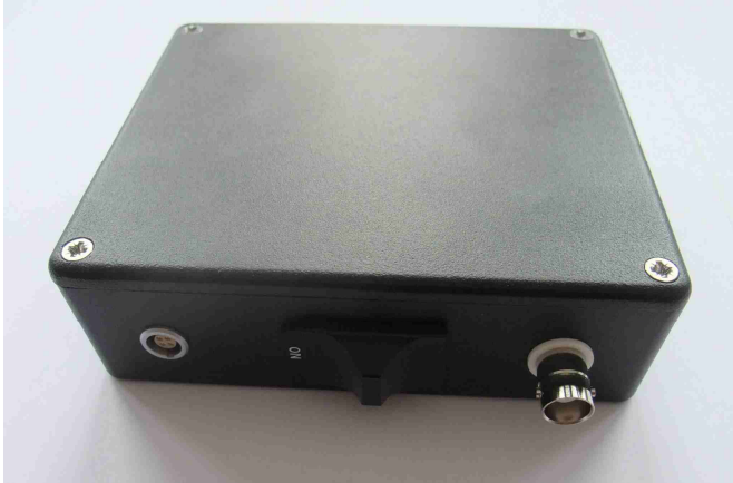
Front view of the power supply +/- 9 V with connector type LEMO FGG 0B 4p, circuit breaker and BNC output signal connector (from left to right)
