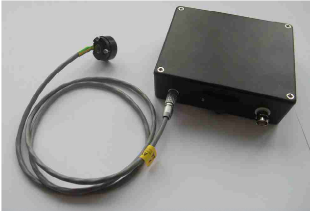
PCA with preamplifier and power supply (here with additional aspheric focusing optical lens for free space laser excitation)
